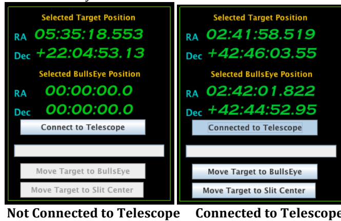
Figure 14 Telescope “control” panel showing the RA-Dec coordinates of the “target” and “bulls-eye” cursors.
