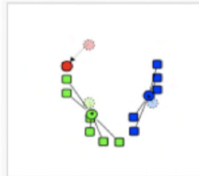
Now the initial randomized points are moved to the center of their respective clusters (the centroids).
