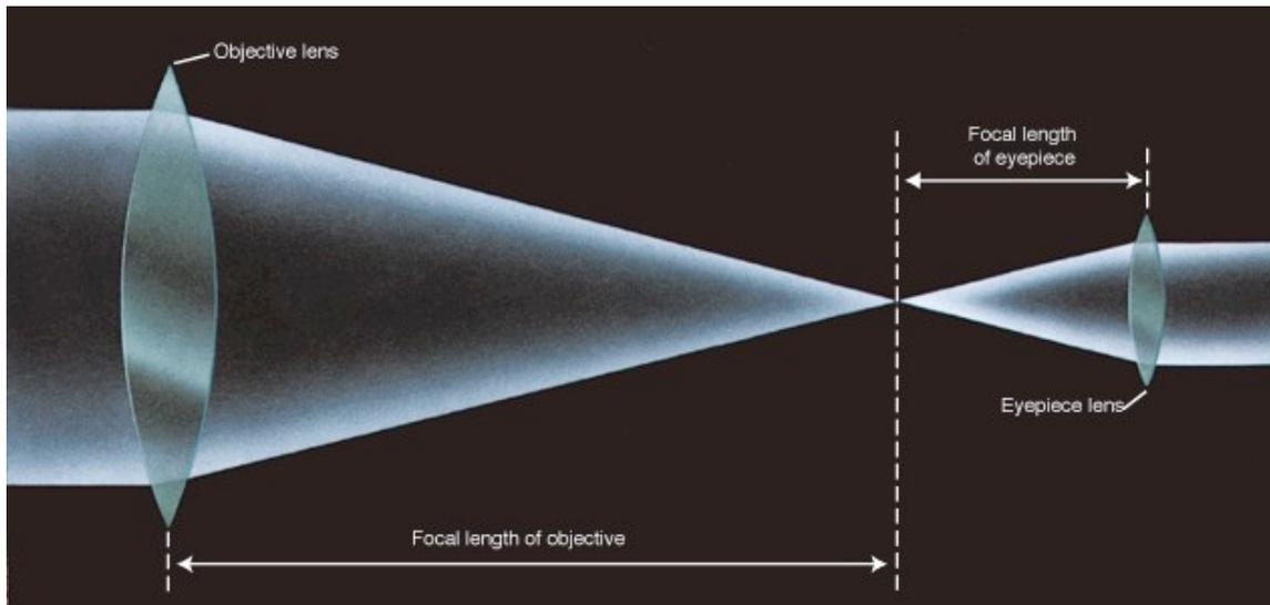
The way it works is quite simple. Light from the star is refracted by its passage through the “Objective Lens” to a point inside the telescope. The light does not stop there! The focus point is simply the point where all the light rays gathered by the objective lens meet. The light keeps going, and is re-refracted by the “Eyepiece Lens” into an image that a human eye can recognize. How much a telescope will magnify an object depends on the “focal length” of each lens.
