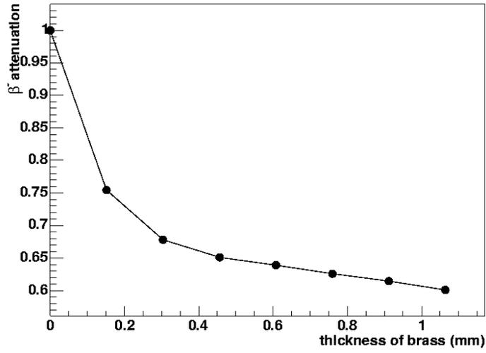
Figure 7: The attenuation in the counting rate of  $\beta^-$  from  $^{90}\text{Sr}$  versus the thickness of brass between the source and the tower.
