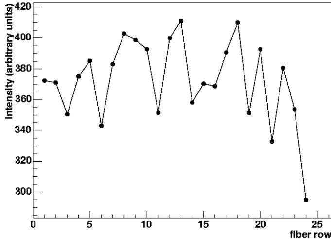
Figure 6: The measured intensity from a stack of ultraviolet LEDs from each row of scintillating fibers.
