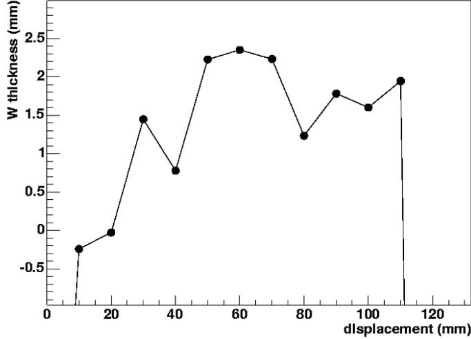
Figure 9: The experimentally determined estimate of the variation in tungsten powder thickness.
