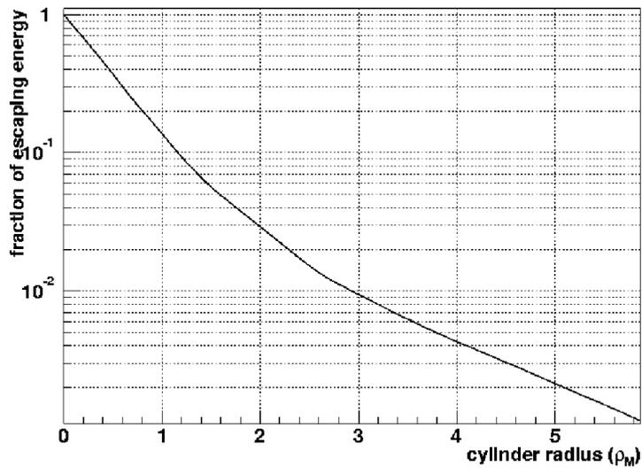
Figure 4: Experimentally determined fraction of energy escaping a long cylinder. Radial units are the Molière radius. Data taken from [4].
