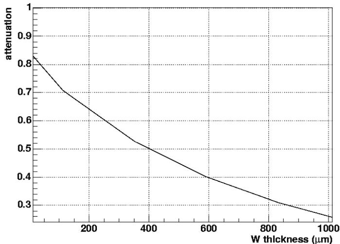
Figure 10: Inferred electron attenuation versus tungsten thickness using data from [4].
