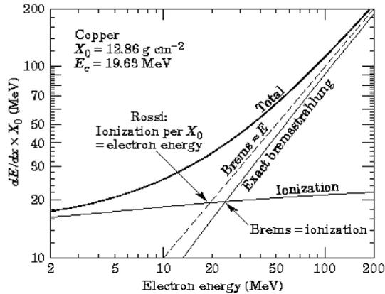
Figure 2: The energy loss of electrons in copper versus kinetic energy. Bremsstrahlung radiation is approximately proportional to the energy of the particle, but the exact relation is also shown. The critical energy is the point at which losses due to Bremsstrahlung radiation are equal to losses due to ionization. Figure taken from [2].
