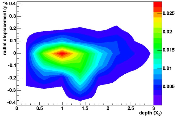
Figure 3: Experimentally determined energy deposition in lead from a 1 GeV electron beam. The contours display the percentage of total deposition. Energy deposition is roughly independent of the absorbing material when plotted in terms of  $X_0$  and  $\rho_M$ . Data taken from [4].
