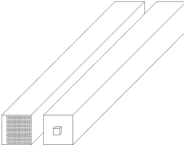
Figure 5: T466 EMC towers. The left tower shows the incident face, where the square scintillating fibers are visible through the mirror. The right tower shows the back face, where the light mixer emerges from the brass container. The PMT abuts this protrusion.
