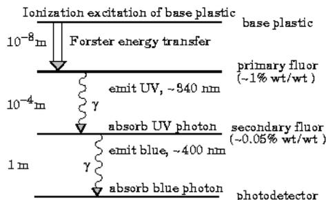
Figure 1: An energy ladder diagram showing the transfer of particle energy to detectable photons in a plastic scintillator. The numbers on the left give the length scale of the energy transfer, and the numbers on the right give the concentration of each fluor by weight. Figure taken from [2].
