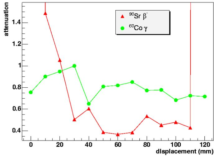
Figure 8: The attenuation in the counting rates from  $^{60}\text{Co}$  and  $^{90}\text{Sr}$  versus longitudinal displacement along the tower.
