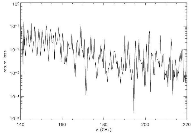
*Fig. 2.4:* The return loss spectrum for the 150 GHz QUaD horn #1, the one used in the 150 GHz spectral testing presented in this thesis.
