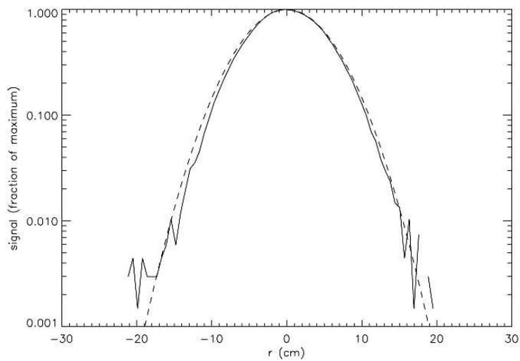
Fig. 4.5: A beam map from the 150 GHz horn #2.
