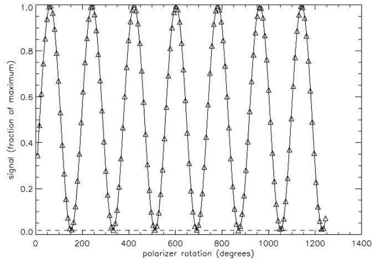
Fig. 3.5: The cross-polarization of PSB 150-21 BOTTOM and its best-fit sine wave. The dashed line is the cross-polar response of this bolometer: 1.81%.
