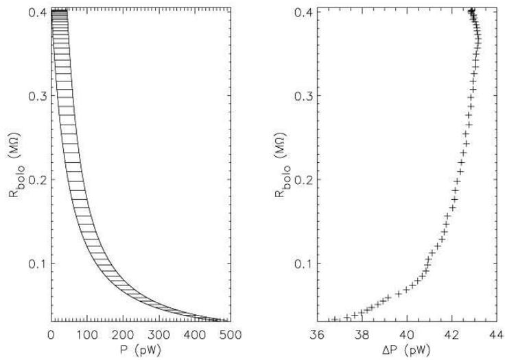
Fig. 2.15: The load curves for PSB 150-21 BOTTOM, for which  $T_{\text{base}} \approx 321$  mK without temperature controlling.
