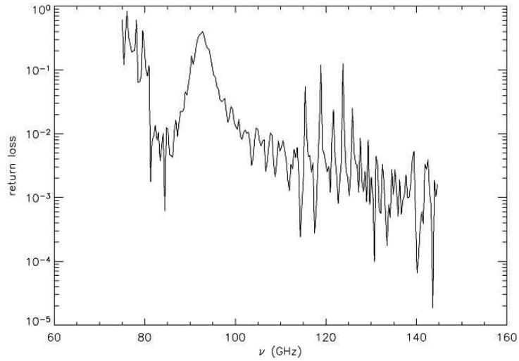
*Fig. 2.3:* The return loss spectrum for the 100 GHz QUaD horn #9, the one used in all of the 100 GHz testing presented in this thesis. The high return loss at 92 GHz may present a problem for this band.
