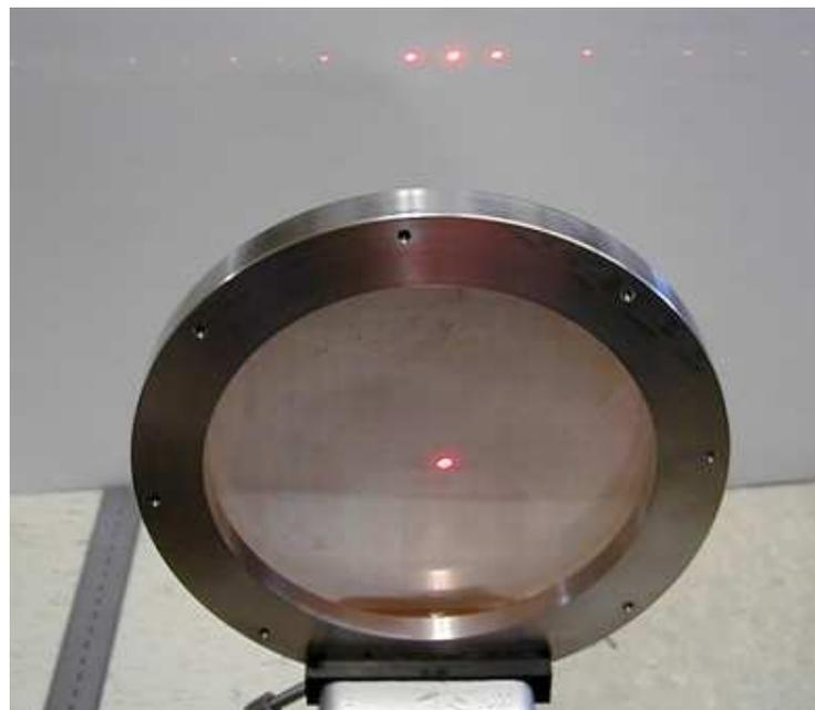
Fig. 3.2: Measuring the polarizer's wire spacing  $d$ .
