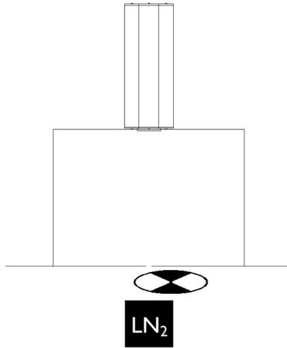
Fig. 4.1: The beam mapper. The aperture, the chopper wheel, and the cold load translate left and right while the dewar remains stationary atop the light-tight, Eccosorb-lined box.
