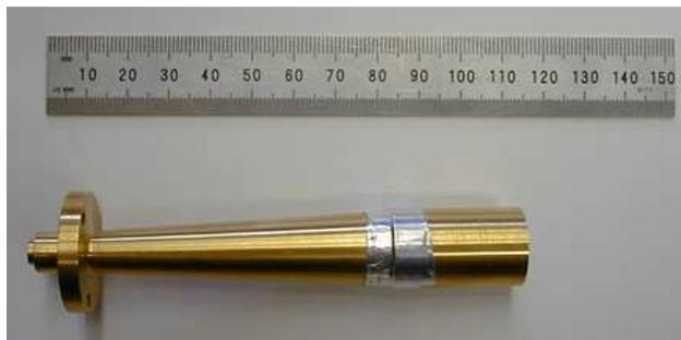
*Fig. 2.2:* A QUA 150 GHz horn shown with its filter cap.
