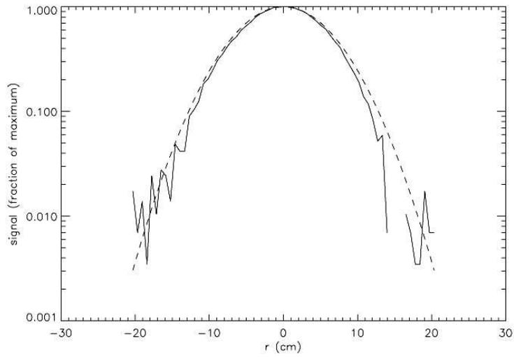
Fig. 4.4: A beam map from the 100 GHz horn #9.
