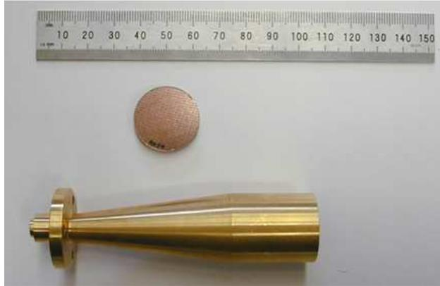
*Fig. 2.1:* A QUA 100 GHz horn shown with an edge filter, described in section 2.1.2.
