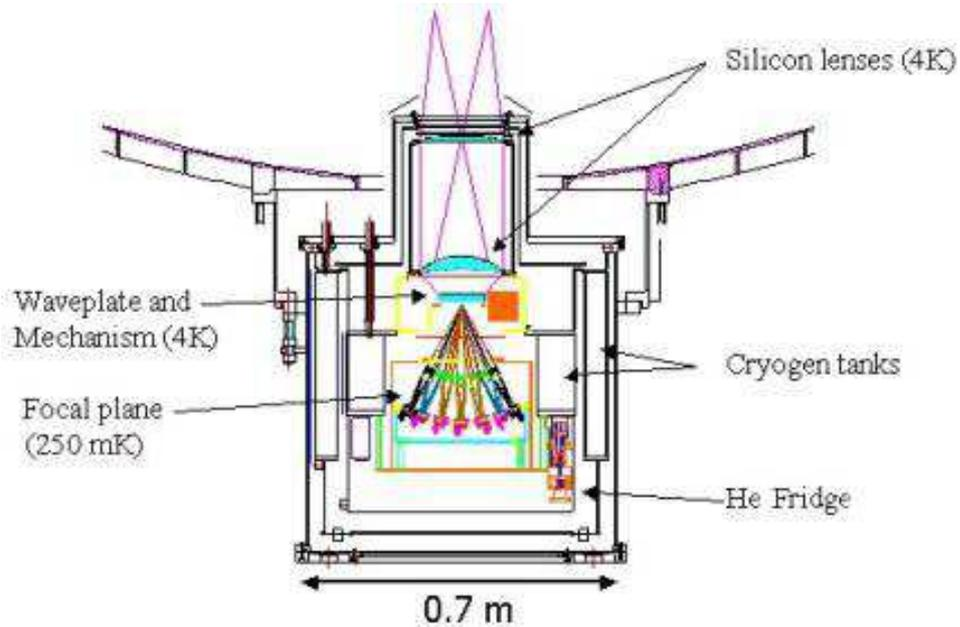
Fig. 1.1: The QUaD receiver on the DASI mount. Ray traces show the path of CMB radiation into the 31 feed horns on the focal plane.
