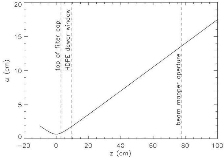
Fig. 4.2:  $\omega$  as a function of displacement from the phase center along the beam axis for a 100 GHz QUaD horn. The dotted lines show the positions of the end of the horn's filter cap, the dewar window, and the beam mapper source aperture.
