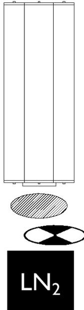
*Fig. 3.3:* The cross-polarization measurement. The dewar looks at a chopped liquid nitrogen cold load through the polarizer. The polarizer rotates in place, and the bolometer signal is recorded for many angles of rotation.
