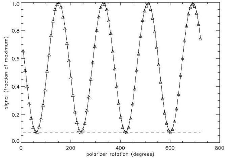
Fig. 3.4: The cross-polarization of PSB 100-14 TOP and its best-fit sine wave. The dashed line is the cross-polar response of this bolometer: 7.50%.
