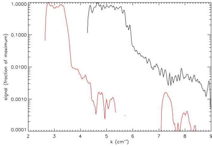
Fig. 2.8: The Fourier transformations of the interferograms from both 100 GHz and 150 GHz configurations. The red line is the Fourier transformation of fig. 2.6 and the black line is the Fourier transformation of fig. 2.7.
