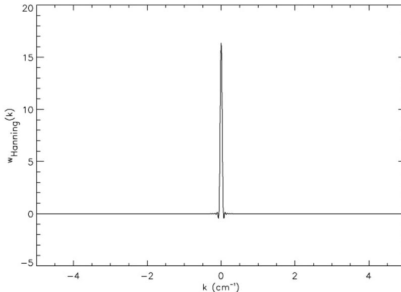
Fig. C.1:  $w_{\text{Hanning}}(k)$  for  $x_{\text{max}} = 16.36$  cm, such as for the 150 GHz interferogram in fig. 2.7.
