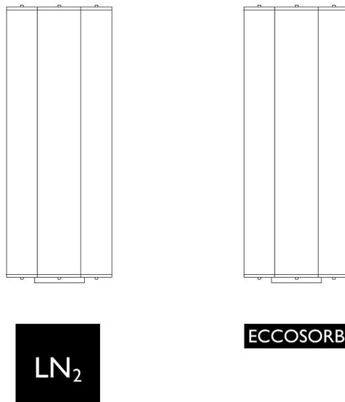
*Fig. 2.11:* The optical efficiency measurement. First, the dewar looks directly at a liquid nitrogen cold load. Then, it looks directly at 300 K Eccosorb. In each configuration, the signal is recorded for the full range of voltage bias on the bolometer.
