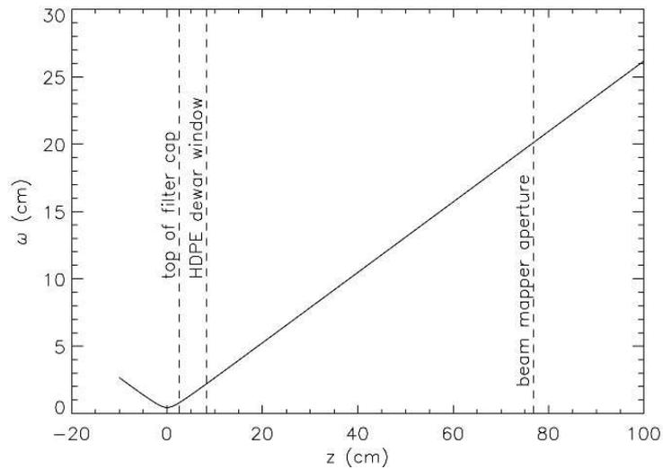
Fig. 4.3:  $\omega$  as a function of  $z$  for a 150 GHz QUaD horn.
