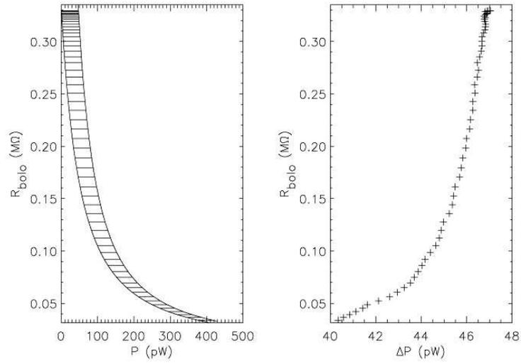
Fig. 2.14: The load curves for PSB 150-21 TOP, for which  $T_{\text{base}} \approx 321$  mK without temperature controlling.
