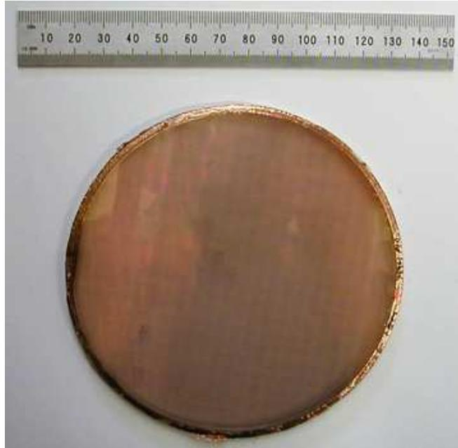
Fig. 3.1: The polarizer.
