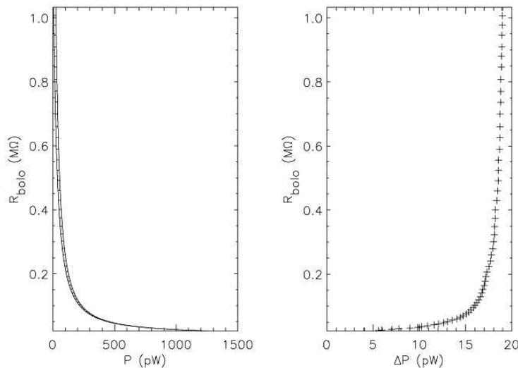
*Fig. 2.13:* The load curves for PSB 100-14 BOTTOM, for which  $T_{\text{base}} = 332 \text{ mK}$  with temperature controlling.
