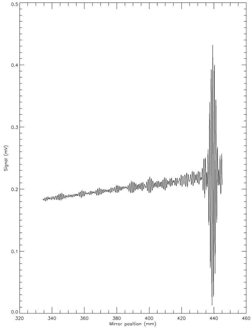
*Fig. 2.7:* The interferogram from the 150 GHz FTS measurement with PSB 150-02 TOP. A mirror misalignment caused the large linear drift.
