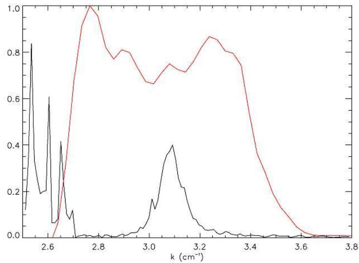
Fig. 2.9: A linear plot of the 100 GHz horn #9's return loss from fig. 2.3 and the transmission function (red) as measured on the FTS from fig. 2.8.
