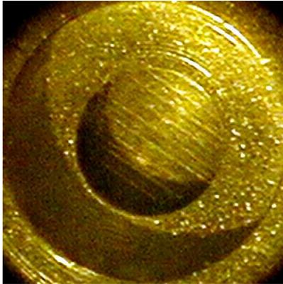
Fig. 1.2: PSB 150-21 magnified 7.5 times. The outer circle accepts the horn mounting flange. The wire mesh is suspended within the inner circle.
