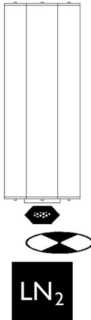
Fig. 2.10: The thick grill filter measurement. The dewar looks at a liquid nitrogen cold load through a filter of small waveguides.
