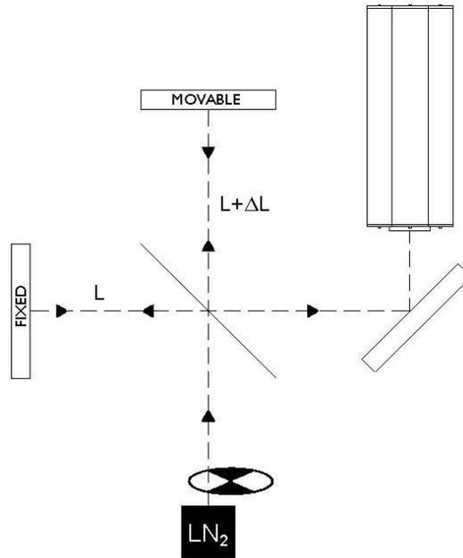
*Fig. 2.5:* The Fourier transform spectrometer. The liquid nitrogen cold load emits 77 K blackbody radiation which the chopper wheel alternates with 300 K blackbody radiation. The beamsplitter sends the in-phase radiation to both a fixed mirror and a movable mirror. The re-combined, interfering radiation reflects into the QUA test bed.
