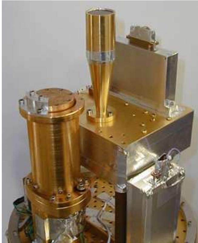
*Fig. 1.4:* The test bed focal plane (the gold plate on which the horn rests) in the 100 GHz configuration. The cylinder on the left is the  $^3\text{He}$  refrigerator, shown here with a aluminum protective immobilizer instead of a copper heat strap to the focal plane. Band-defining filters cap the 100 GHz feed horn at the center of the focal plane. The PSB mounts to the bottom of the horn, under the gold plate. The box to the right of the horn houses the load resistors.
