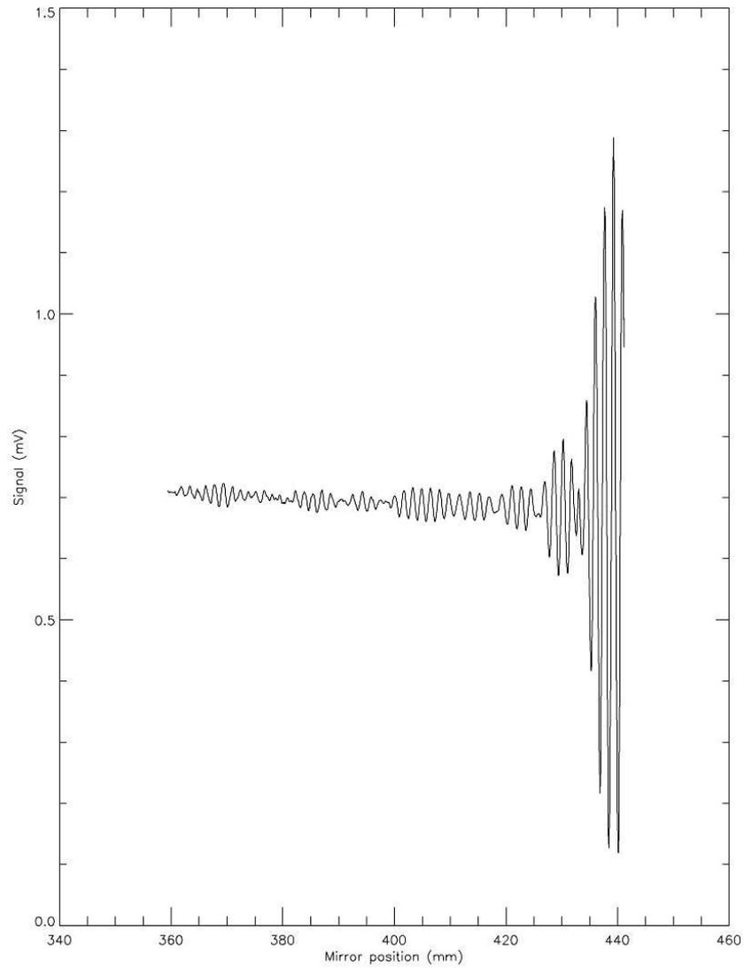
*Fig. 2.6:* The interferogram from the 100 GHz FTS measurement with PSB 100-14 TOP.
