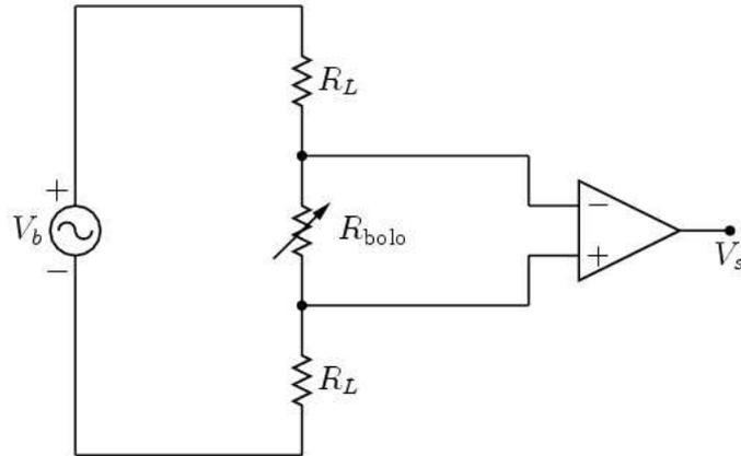
Fig. 1.3: A simplified circuit diagram of the bolometer electronics. The voltage  $V_b$ , shown here as AC, biases the bolometer with temperature-dependent resistance  $R_{\text{bolo}}$  through the load resistors  $R_L$ . A differential amplifier measures the voltage across the bolometer, called the signal voltage  $V_s$ .
