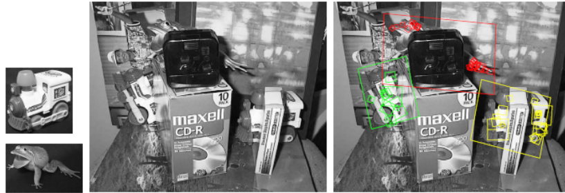
Figure 12: The training images for two objects are shown on the left. These can be recognized in a cluttered image with extensive occlusion, shown in the middle. The results of recognition are shown on the right. A parallelogram is drawn around each recognized object showing the boundaries of the original training image under the affine transformation solved for during recognition. Smaller squares indicate the keypoints that were used for recognition.
