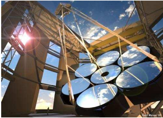
FIG. 10.— Artist conception of the design for one of the future giant telescopes that could probe the first generation of galaxies from the ground. The Giant Magellan Telescope (GMT) will contain seven mirrors (each 8.4 meter in diameter) and will have the resolving power equivalent to a 24.5 meter (80 foot) primary mirror. For more details see http://www.gmto.org/
