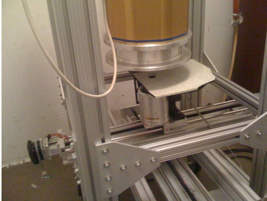
Figure 6.10. Chopped thermal load used for pattern measurements. We extended the 300K surface defining the aperture with more eccosorb than shown to completely block the chopping wheel everywhere except the aperture.
