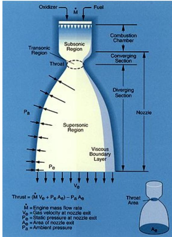
FIGURE 1. A typical nozzle and associated terminology.
