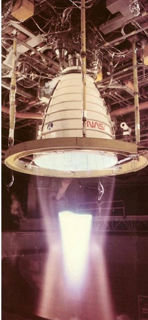
FIGURE 5. SSME Nozzle at sea-level pressure. The shape of the plume varies with the ambient pressure. Next time you see the Shuttle being launched look for the change in shape (cylindrical with Mach disk at launch; gradually the diameter of the cylinder should increase and the Mach disk should disappear; finally the plume should look a cupola.)
