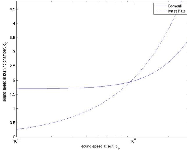
FIGURE 2. SSEM: The speed of sound at the exhaust,  $c_e$ , versus the speed of sound in the burning chamber,  $c_0$ . The curves are for the parameters relevant to the SSEM. The solid curve is the square root of the right side of Equation 21 and the dotted line is the square root of the right side of the same Equation.
