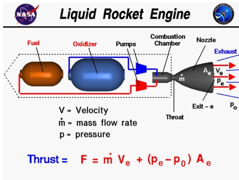
FIGURE 4. Cartoon view of a liquid engine rocket.
