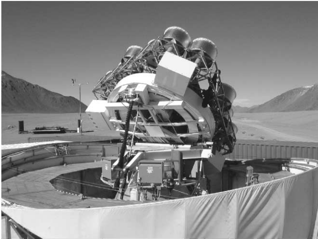
Fig. 3.—Rear view of the CBI. The struts underneath the elevation platform support the parallactic angle cable wrap and the elevation drive motor, which is at the top of the ballscrew. The ballscrew nut is attached to the forks at the back of the azimuth platform. The cables and hoses at the bottom of the elevation platform are part of the elevation cable wrap, which is just behind the elevation axis. The three white boxes attached to the back of the antenna platform contain the signal processing and drive control electronics and uninterruptible power supplies. The 15 cm refractor used for pointing measurements is to the right of the uppermost electronics box.
