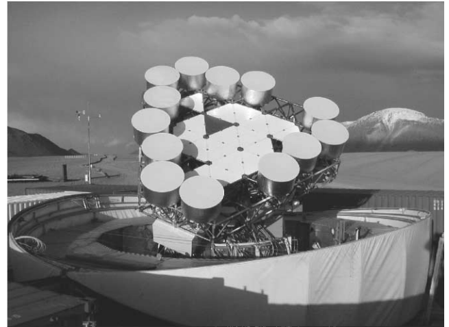
Fig. 4.—Front view of the CBI with the antennas in a ring configuration. This permits easy access to the receivers and was used for testing the CBI and for our first measurements of the power spectrum of CMBR fluctuations. The helium compressors for the refrigerators are at the front of the telescope, on a frame attached to the azimuth platform.
