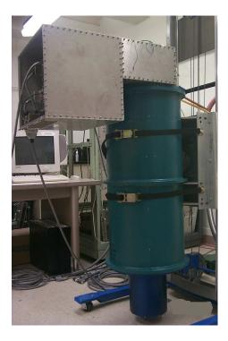
Figure 2.7: Photograph of the Bolocam dewar in the lab at Caltech. Note the large RF-tight enclosure on top of the dewar, which contains the first stage amplifiers.
