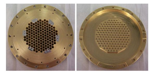
Figure 2.9: Left: a photon's-eye view of the horn-plate used for 2.1 mm observations. Right: the view from the bolometer of the same horn-plate.
