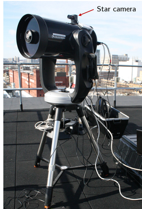
Fig. 3 Portable Telescope for Lasercom (PorTeL) deployed on the roof of MIT building 37 in Cambridge, Massachusetts. The star camera can be seen mounted on top of the telescope.
